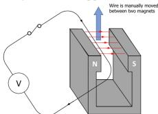
In both the experiments, emf and current is induced due to the change in the magnetic flux linking through the coil or wire.
